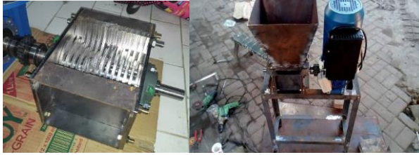
Figure 6. Cutter box assembly (left) and final assembly (right)
