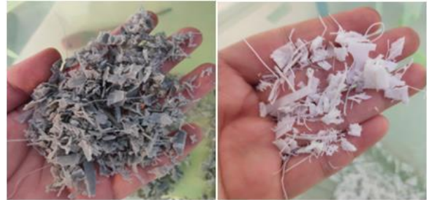
Figure 10. Unfiltered crushing of ABS(left) and PLA(right).
