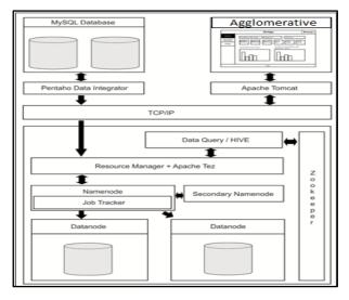
Figure 2. System architecture
